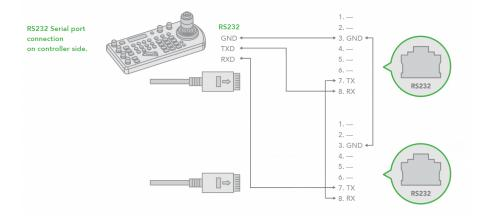
b. Use a CAT5/6 network cable (T-568B standard pinout) to make an RS232 connection by following the pin definition below:
