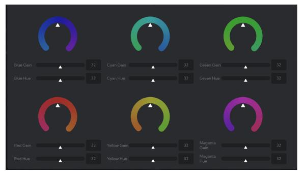
The Color Matrix features 64 levels of adjustment of Gain (Intensity) and Hue (offset) across six color sections, Red, Green, Blue, Cyan, Magenta and Yellow, and allows individual fine-tuning of each of these without affecting the response of other color components.
